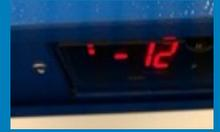
Check back at least 60 minutes later to see if temperature has regulated. If frozen cups are warmer than  $-15^{\circ}\text{C}$ , the blender may not blend correctly or at all. Extra cold cups ( $-18^{\circ}\text{C}$  and below) will cause the blender to take longer to blend and will eventually shorten the life of the blender and/or blender parts and may cause damage.
