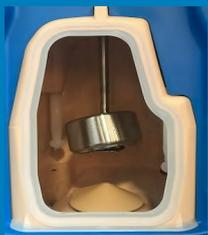
1) Open the front door and perform a visual inspection to verify the surfaces are clean and check for any debris in chamber (lids).
